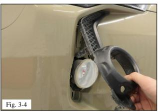
(i) Gently bend the bezel back exposing the fog lamp splash shield mounting tabs (Fig. 3-4).
