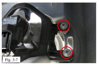
(m) Using #2 Phillips screwdriver, remove the (2) mounting screws (Fig. 3-7).
