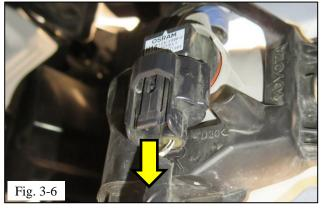
(l) Disconnect fog lamp connector by pressing the release button and pulling downward (Fig. 3-6).
